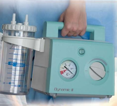
Dynamic II is a compact modern medical device for efficient suction, suitable for wards and ICUs as well as for homecare. A double piston oil-free vacuum pump guarantees a dynamic suction output (20 I/min) and it's completely maintenance free. By using the suction regulator it's possible to control the vacuum level in the range of 0-80 kPa. The value is monitored by a vacuum gauge.
