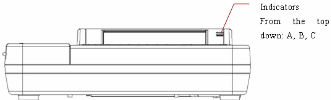
Figure 2-4 SE-1200 Express Front Panel
