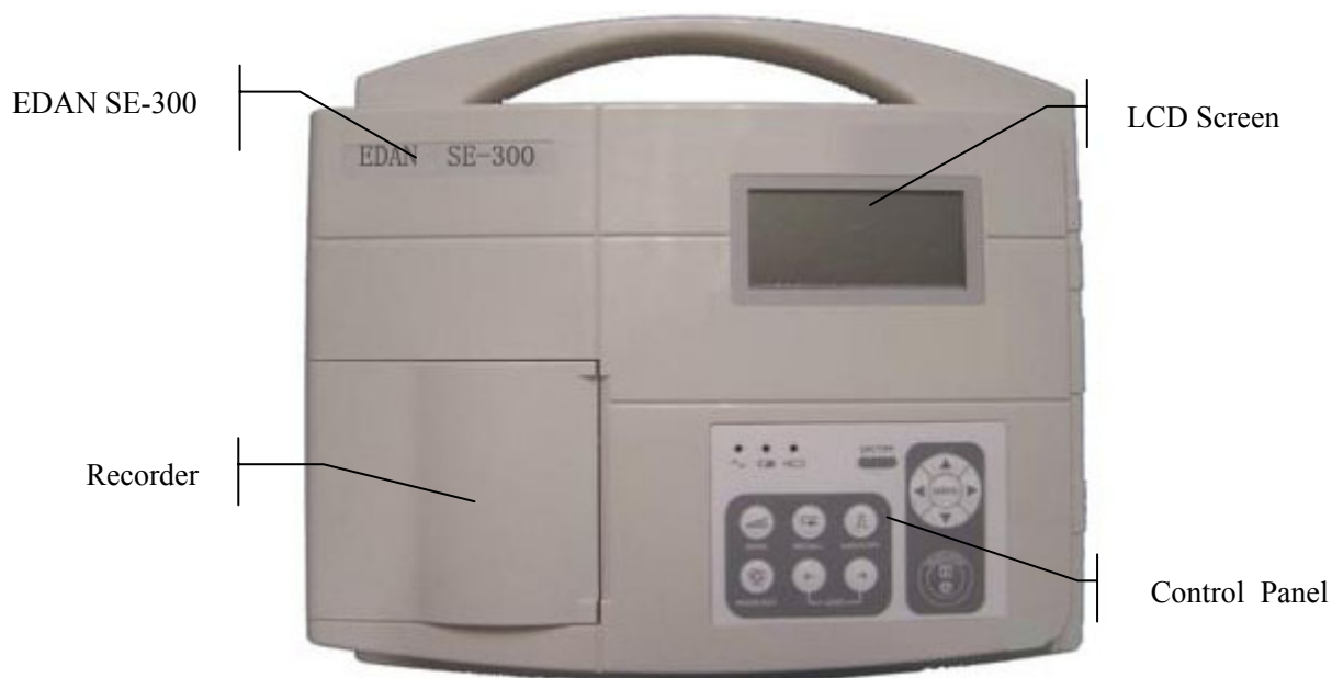
Figure 2-2 SE-300A (the device with the LCD screen of 192×64 dot single color)
